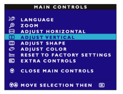
3) Press the **low** button. The ADJUST VERTICAL window appears. POSITION should be highlighted.
